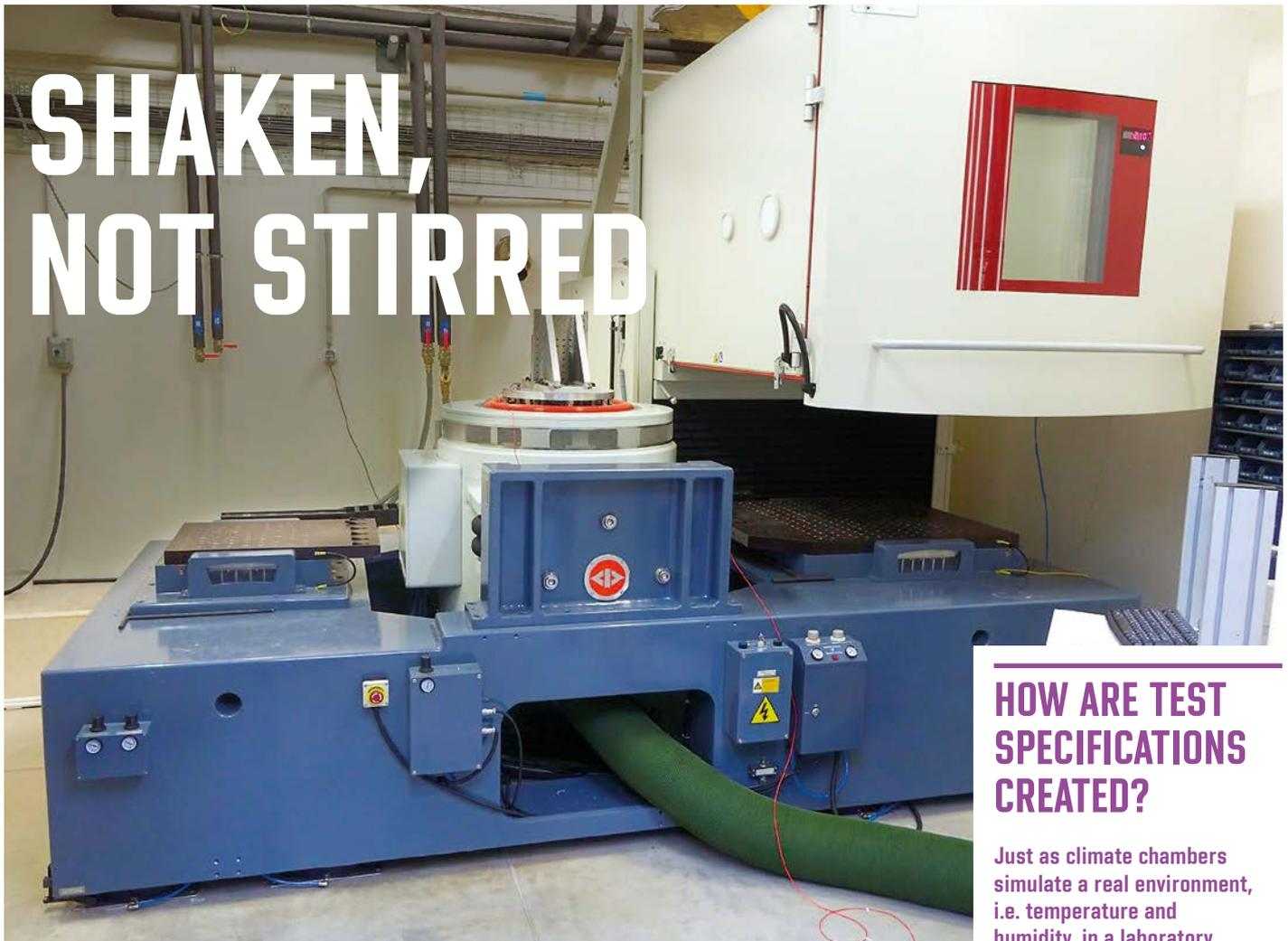
**Yes, it is a shaker, but not just any shaker. This one is used to test the vibration of, for example, automotive parts.**
